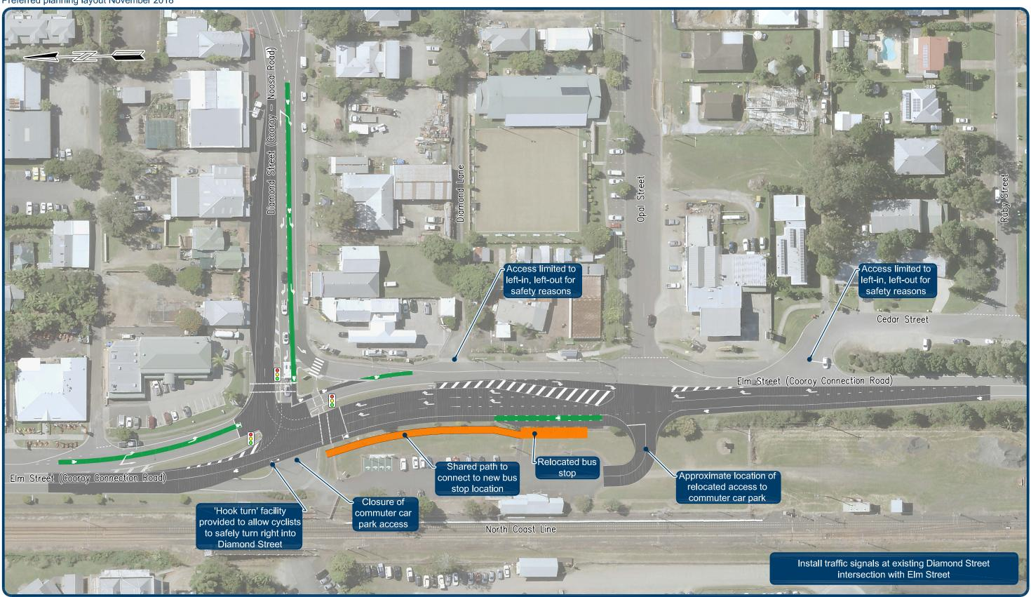
The preferred option will involve upgrading the current arrangements by introducing traffic signals to control traffic movements and provide safe signalised crossing opportunities for active transport users. This option provides increased capacity by providing two right turn lanes from Elm Street into Diamond Street and caters for forecast traffic growth well into the future.
