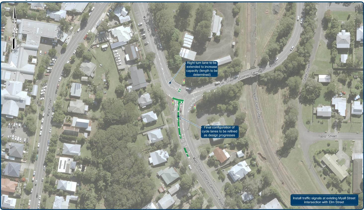
The preferred option will involve upgrading the current arrangements by introducing traffic signals to control traffic movements and provide safer signalised crossing opportunities for active transport users.
